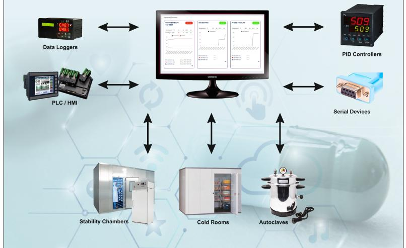
21 CFR Part 11 Data Logging Application for Temperature, Humidity, or any other Environmental Parameters
